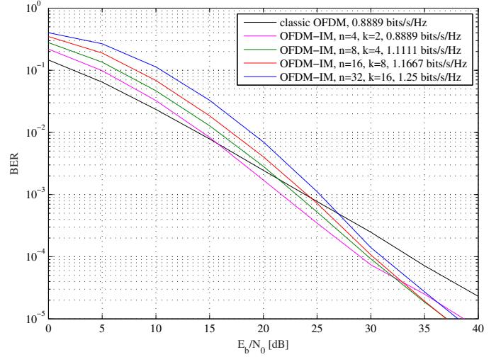
Fig. 7. BER performance of OFDM-IM with different configurations.
