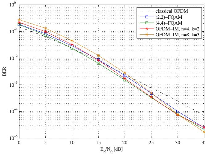
Fig. 9. BER of schemes with spectral efficiency 0.8889 bits/s/Hz.
