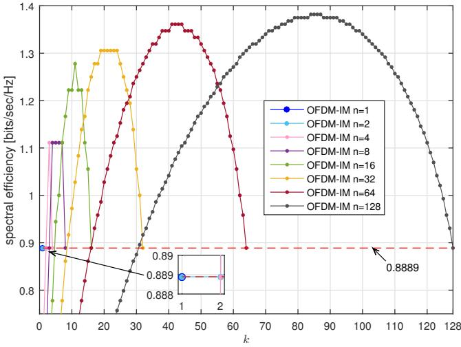
Fig. 5. Spectral efficiency of OFDM-IM.
