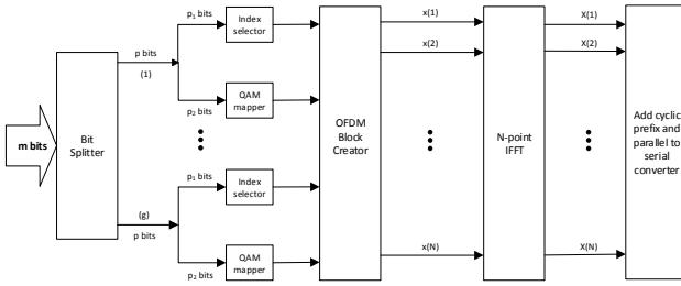
Fig. 1. Block diagram of the OFDM-IM transmitter.
