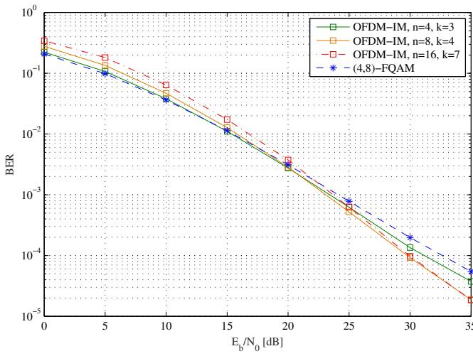
Fig. 10. BER of schemes with spectral efficiency 1.1111 bits/s/Hz.
