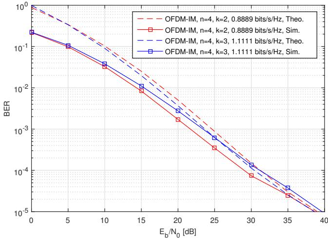
Fig. 3. Theoretical and simulation results for the BER of OFDM-IM.
