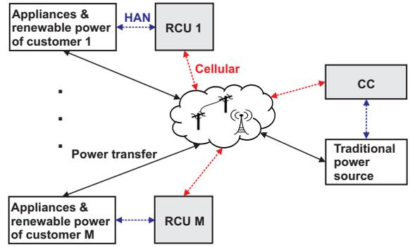
Fig. 1. System model composed of a traditional power source, users with residential control units, cellular communication network and power distribution network.
