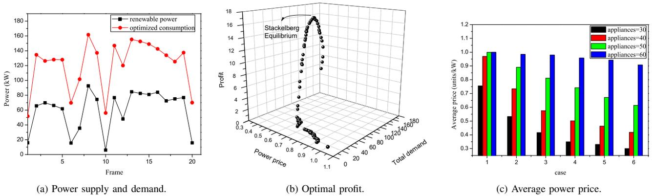
Fig. 2. Performance of the proposed DSM schemes in demand curtailment, operator's profit and power price.
