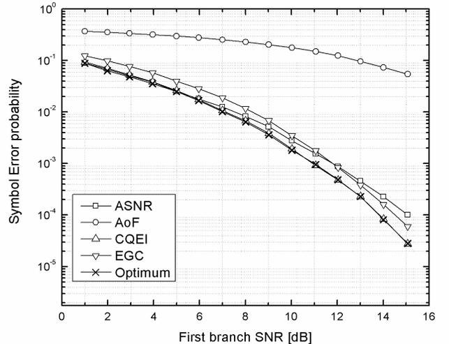
Figure 4: The performance of the EGC receiver when various criteria employed, compared to an  $L = 5$  EGC receiver for a BPSK communication system performing over Nakagami- $m$  fading, assuming non-i.i.d branches ( $d = 2$ ,  $m_1 = 1.2$ ,  $m_2 = 2$ ,  $m_3 = 3.1$ ,  $m_4 = 2.2$ ,  $m_5 = 3.0$ ).
