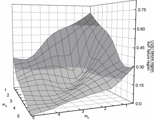
Figure 2: The ratio of the AoF failure region to the CQEI failure region, as a function of the Nakagami- $m$  parameters, for a 4-PSK communication system.
