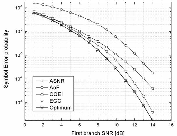
Figure 3: The performance of the EGC receiver when various criteria employed, compared to an  $L = 5$  EGC receiver for a BPSK communication system performing over Nakagami- $m$  fading, assuming non-i.i.d branches ( $d = 1$ ,  $m_1 = 1.5$ ,  $m_2 = 2$ ,  $m_3 = 2.5$ ,  $m_4 = 3.2$ ,  $m_5 = 1.3$ ).
