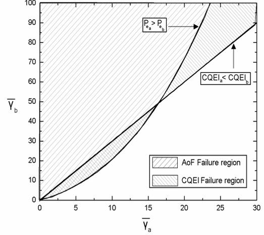
Figure 1: The failure region of the AoF, compared with the failure region of the CQEI, assuming two Nakagami- $m$  channels ( $m_a = 4$ ,  $m_b = 2$ ) and a 4-PSK communication system.
