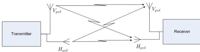
Fig. 3. Illustration of polarization diversity system with dual-polarized transmit and receive antenna.
