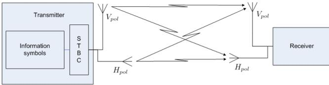
Fig. 7. Dual-polarization transmit-receive system employing STBC encoding.
