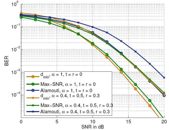
Fig. 9. Comparison between the ideal  $2 \times 2$  MIMO and a realistic case [Vrigneau et al, 15]<sup>1</sup>.
