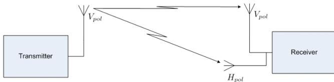
Fig. 2. Receive polarization diversity system.
