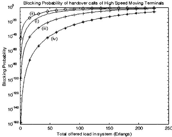
Fig. 2. Handoff blocking probability of HSMT against total offered traffic load in the system. (i) Architecture with no Umbrella Layer and  $C_s = 120$ ,  $C = 40$ . (ii) Proposed Architecture with Umbrella Layer and  $C_s = 120$ ,  $C_u = 24$ ,  $C = 32$ . (iii) Proposed Architecture with Umbrella Layer and  $C_s = 120$ ,  $C_u = 48$ ,  $C = 24$ . (iv) Proposed Architecture with Umbrella Layer and  $C_s = 120$ ,  $C_u = 72$ ,  $C = 16$ .
