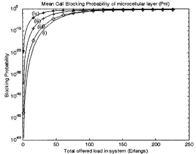
Fig. 3. Mean call blocking probability of the microcellular layer ( $P_{nl}$ ), against total offered traffic load in the system. (i) Architecture with no Umbrella Layer and  $C_s = 120$ ,  $C = 40$ . (ii) Proposed Architecture with Umbrella Layer and  $C_s = 120$ ,  $C_u = 24$ ,  $C = 32$ . (iii) Proposed Architecture with Umbrella Layer and  $C_s = 120$ ,  $C_u = 48$ ,  $C = 24$ . (iv) Proposed Architecture with Umbrella Layer and  $C_s = 120$ ,  $C_u = 72$ ,  $C = 16$ .
