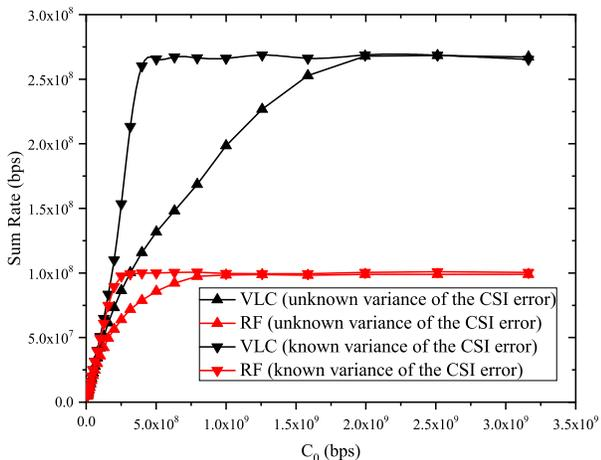
Fig. 5. Sum Rate vs Backhaul Capacity  $C_0$  for  $\alpha = 0.5$  assuming imperfect CSI with  $\rho_{\text{VLC}} = \rho_{\text{RF}} = 0.99$ .
