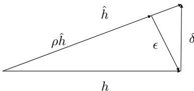
Fig. 2. Orthogonality principle of channel estimation error.
