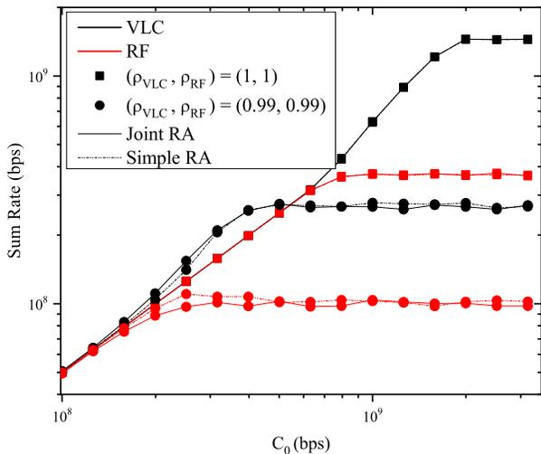
Fig. 4. Comparison between Joint RA and Simple RA in terms of Sum Rate vs Backhaul Capacity  $C_0$  for  $\alpha = 0.5$ .
