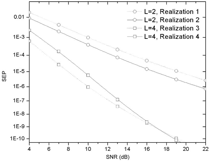
Fig. 2. SEP of DF cooperative diversity versus the average SNR for the case of two and four available relays, assuming BPSK modulation and two different channel realizations per case.
