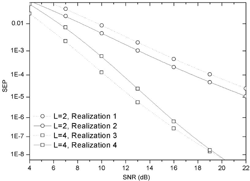
Fig. 3. SEP of DF cooperative diversity versus the average SNR for the case of two and four available relays, assuming QPSK modulation and two different channel realizations per case.
