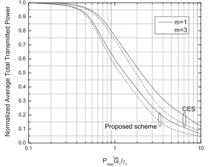
Fig. 3. Average total transmitting power versus  $P_{\max} \bar{G}_1 / \gamma_t$ , for the conventional equi-power scheme (CES) and the proposed scheme in i.n.i.d. Nakagami- $m$  fading with exponential profile, for  $L = 3$ .
