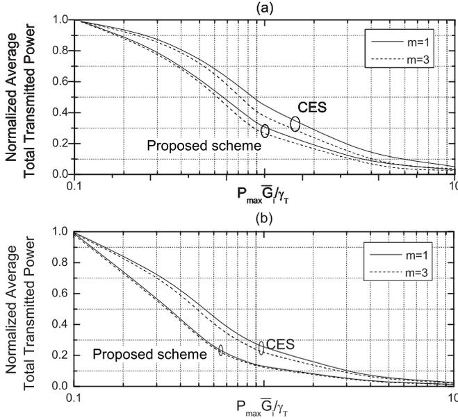
Fig. 2. Average total transmitting power versus  $P_{\max} \bar{G}_i / \gamma_t$ , for the conventional equi-power scheme (CES) and the proposed scheme in i.i.d. Nakagami- $m$  fading for (a)  $L = 3$  and (b)  $L = 5$ .
